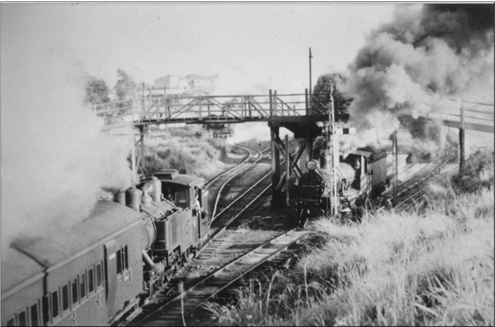
Manly Photo No 12 Transport – Rail - the “steamy” days of Manly Station are recalled in this view of some three steam engines at the station at the same time – one is arriving from Lota, one is waiting for the Lota train to move on so it may proceed to the turntable to be reversed for its next journey to Brisbane, and the third is just visible under the footbridge being turned about on the turntable.
