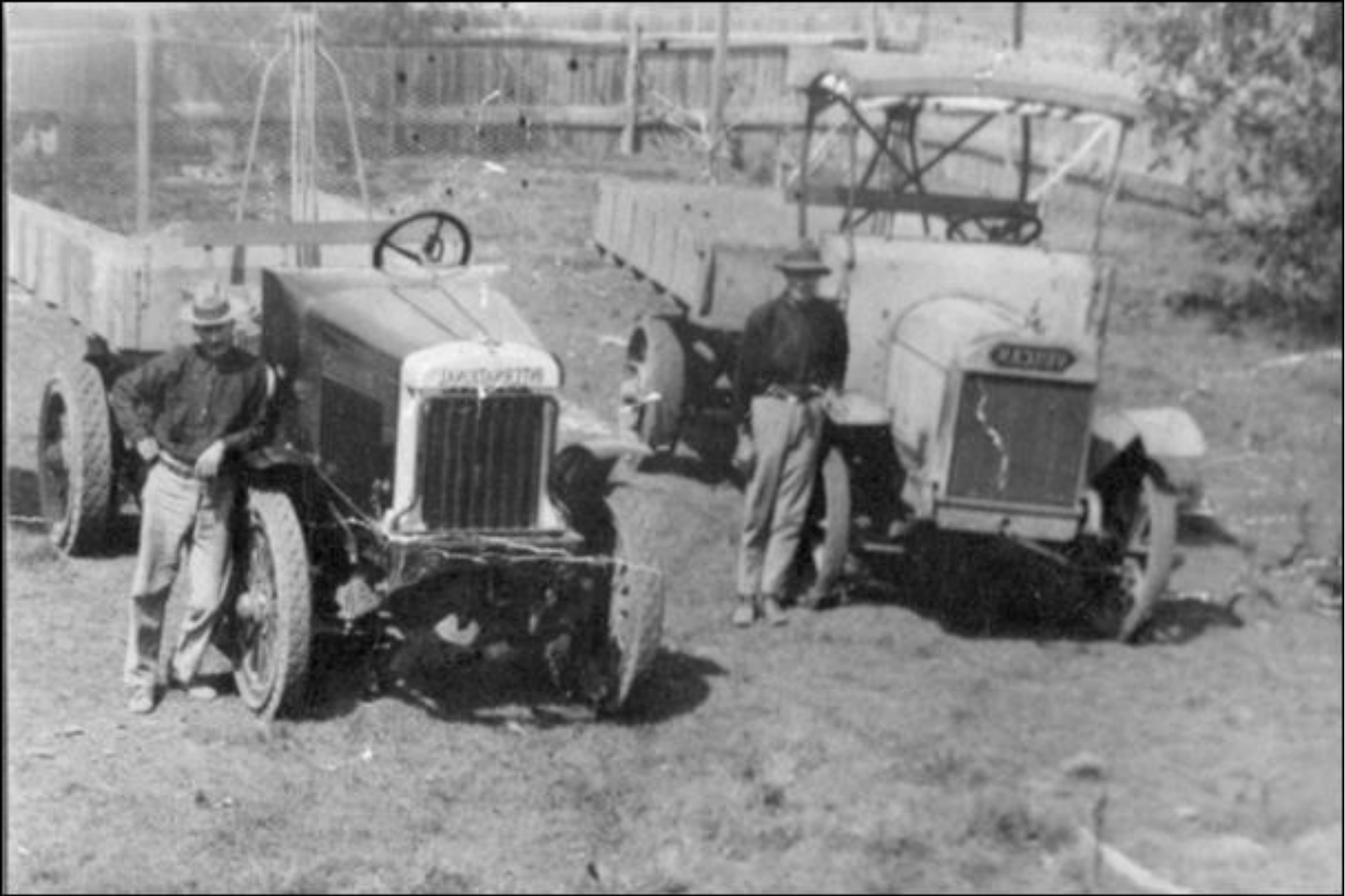
Wynnum – 1927 Photo No 261 Transport – Road - Joe Pyle and Son's trucks were under contract to the infant Brisbane City Council for road building and other jobs in Wynnum – take note of the iron wheels and the solid rubber tires – no need to worry about a puncture – tip trays were fitted on these early vehicles Myrtle Beitz, August 2004
